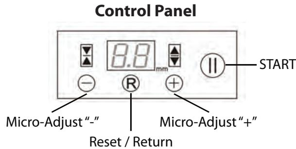
1. Different brands of wires might be produced with different materials and/or different wire forming machines, thus having different flexibilities (wire closing memories). To ensure a perfect wire closing result with all types & brands of wires, your FlexiCloser is equipped with a Micro-Adjust Feature.
