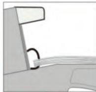
3. Make sure the wire is horizontally-centered in the Wire Closer Channel. Never place wires (especially short wires) on only one side of the machine.
